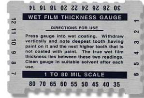
Coverage should average 50 square feet per gallon at 20 mils thickness on flat surfaces. Coverage should average approximately 80 square feet a gallon on smooth metal surfaces at 13 WMT. 13-15 mil coats of ThermaCote® will dry in 2 hours at 70° F in low humidity atmospheres (less than 5,000 feet above sea level).
